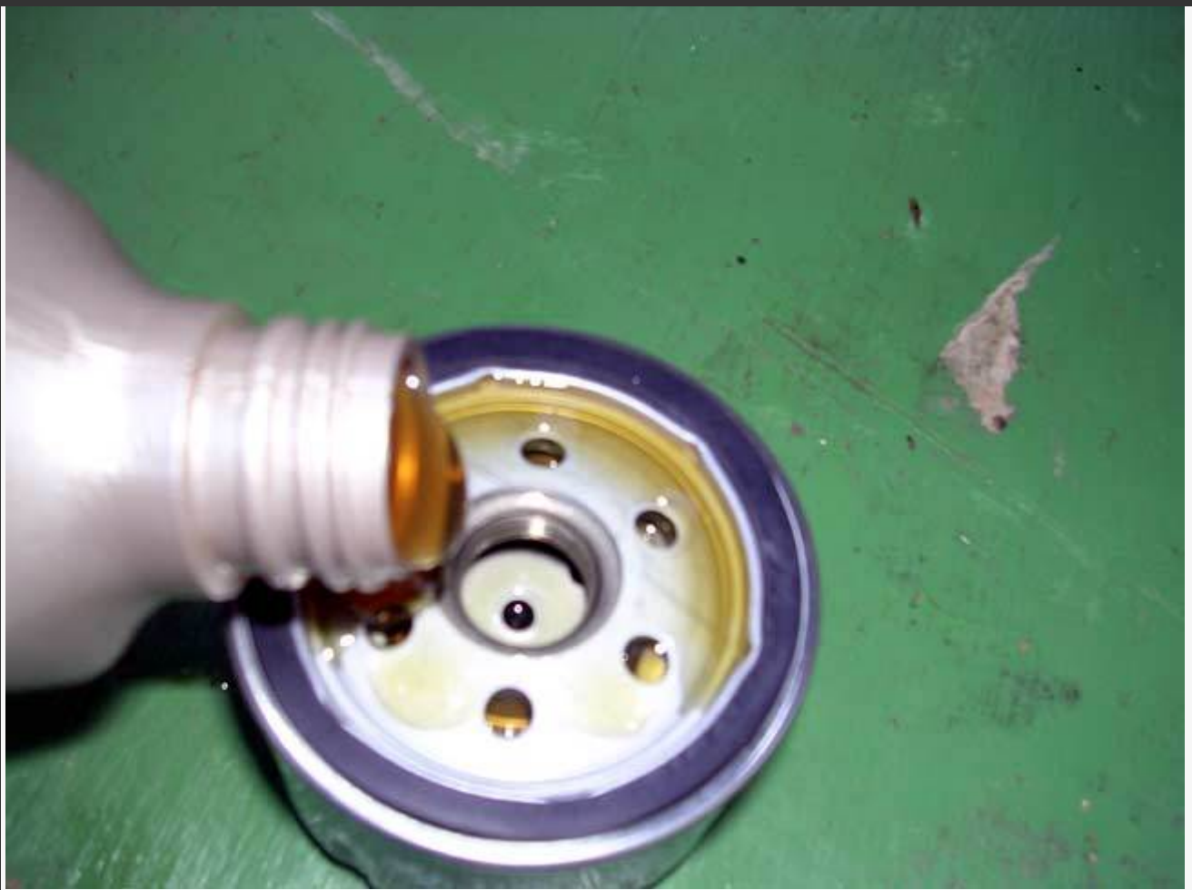
I usually fill the filter first, using a little oil on the rubber o-ring to help seal it, and keep it from sticking next time.
