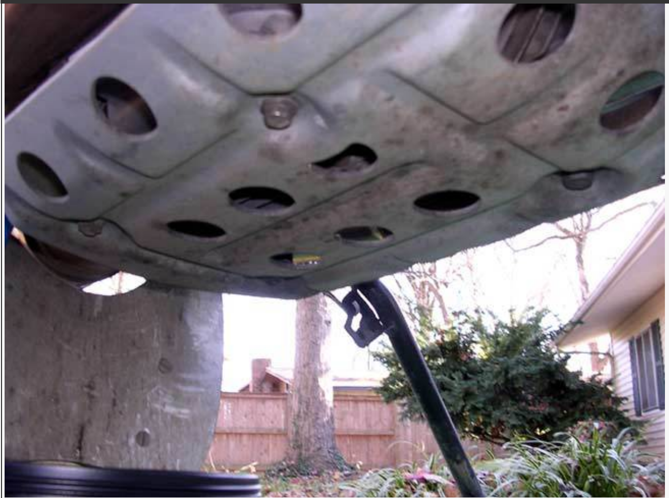
On the GS remove the bash plate.
