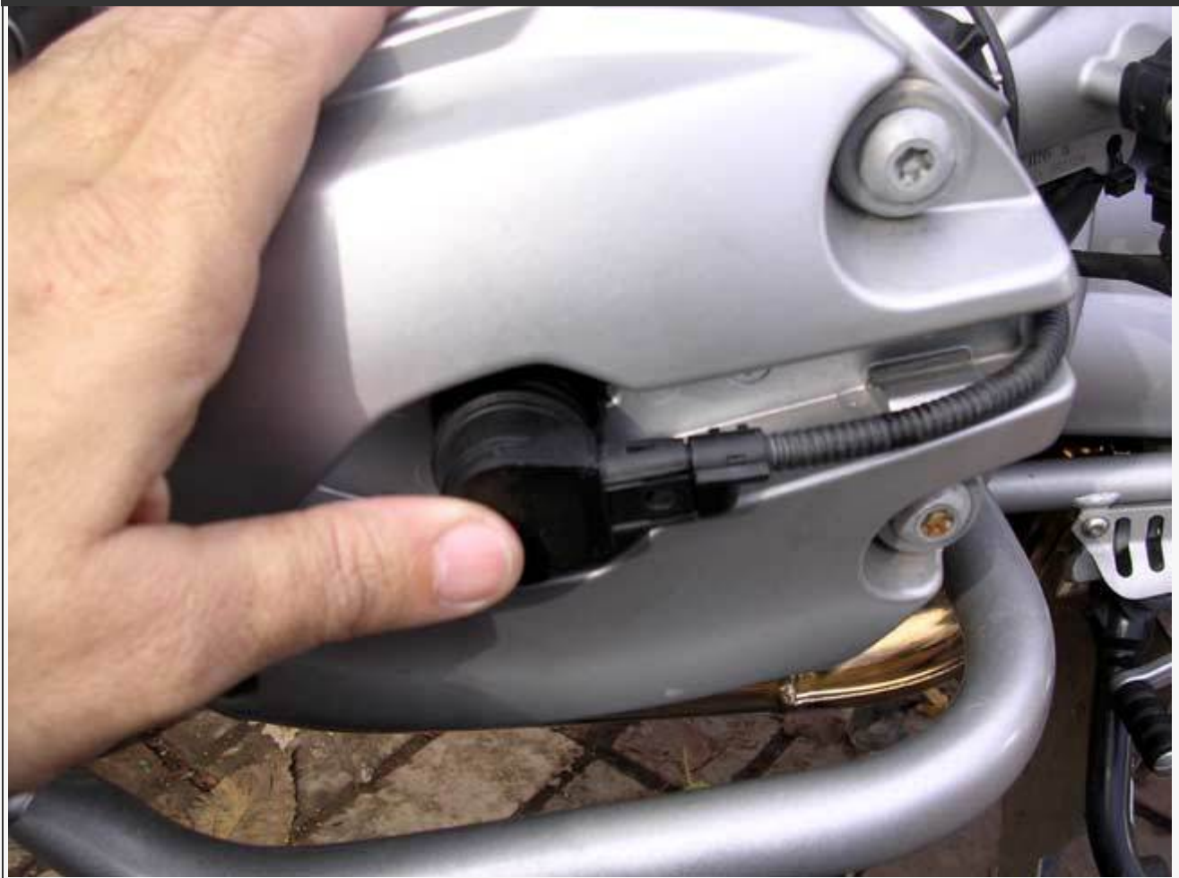
Place the plug wire in place.
