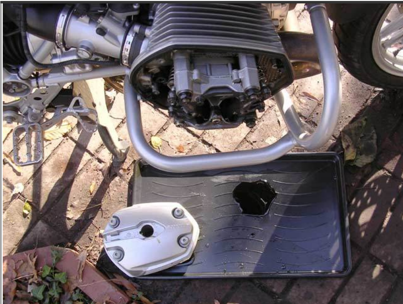
The Valve Cover removed. The drip pan is a cheap plastic one from the dollar store. I have been known to use a cookie sheet. Note the small amount of oil. That is all that normally falls out when removing the valve cover.
