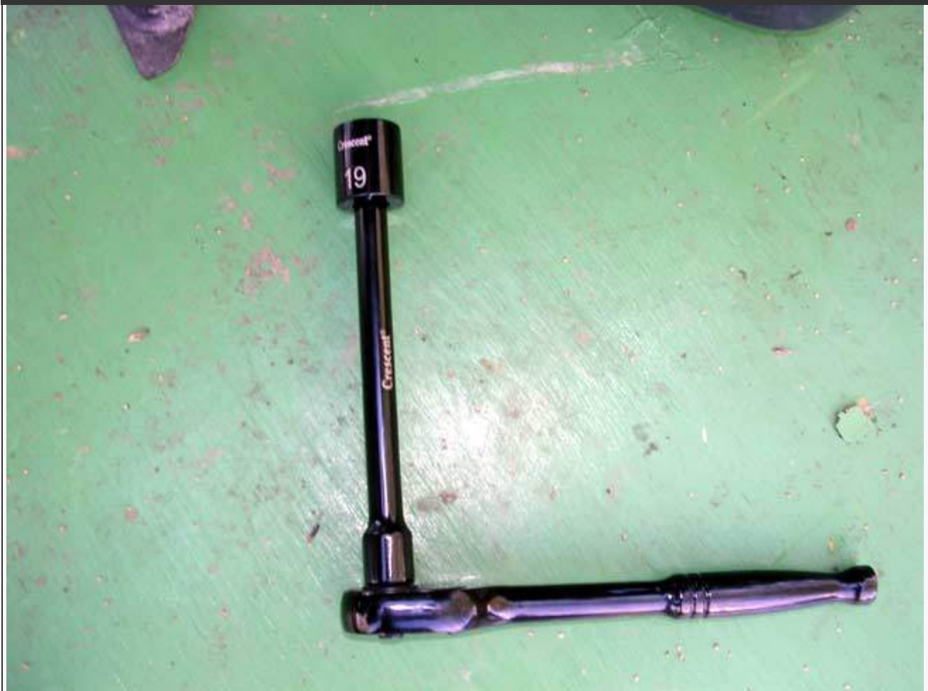
The trans drain takes a 19mm socket. Just loosen and remove the bolt
