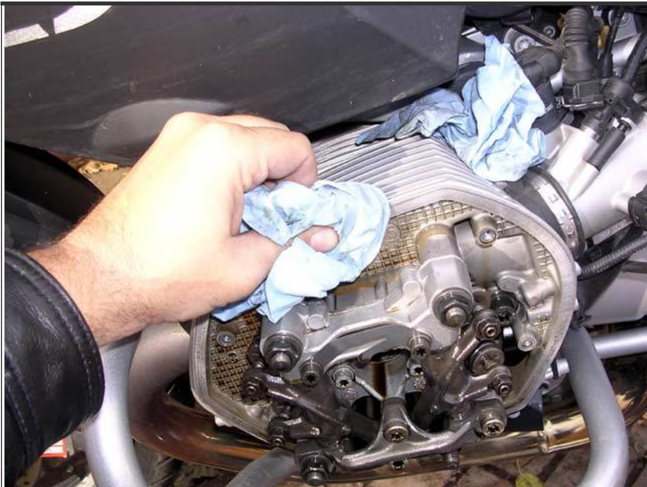
Clean the head surface. Then place the gasket back on the head.
