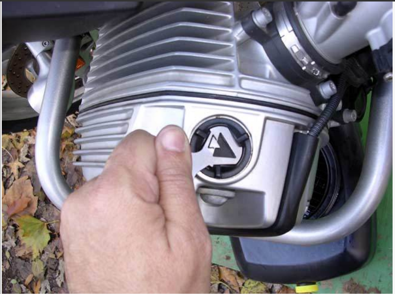
Remove the filler cap on the engine. I use a TT, I think, filler cap removal tool.
