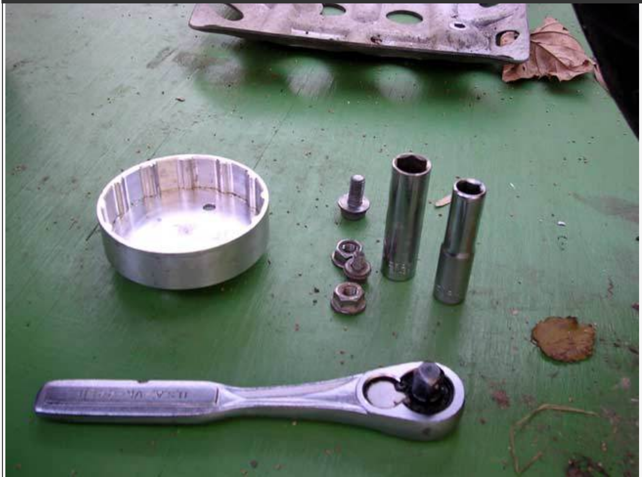
It takes a 13mm socket, and a 10mm socket. Simply loosen the nuts, and the 10mm bolt, and the plate will fall off.
