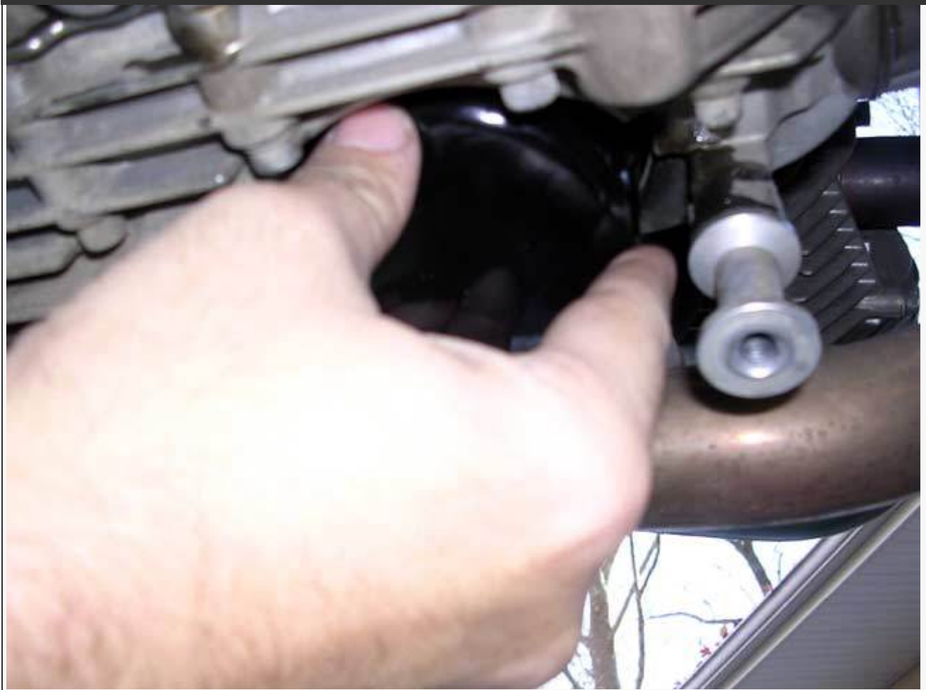
Install the filter by hand first.
