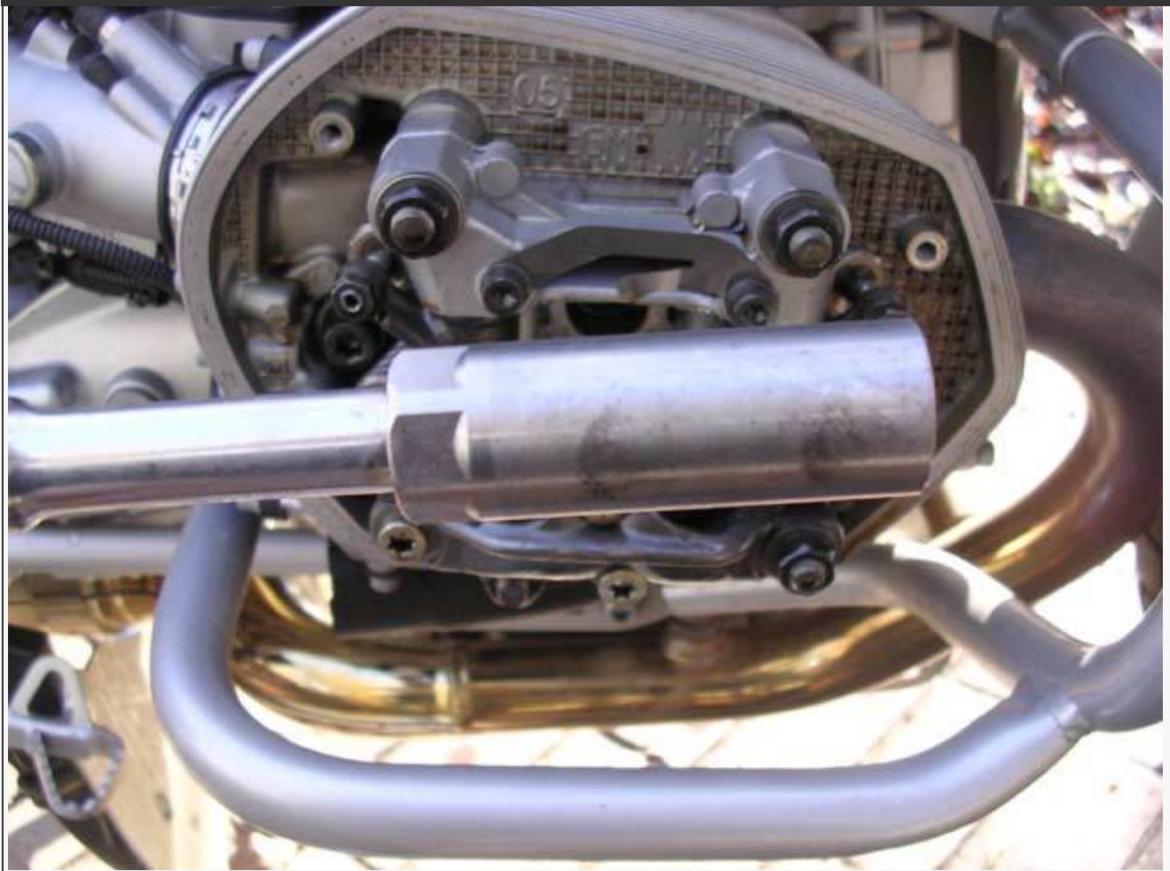
This is a special plug wrench. Actually a trimmed down Craftsman. It makes it easier to get the socket in and out.
